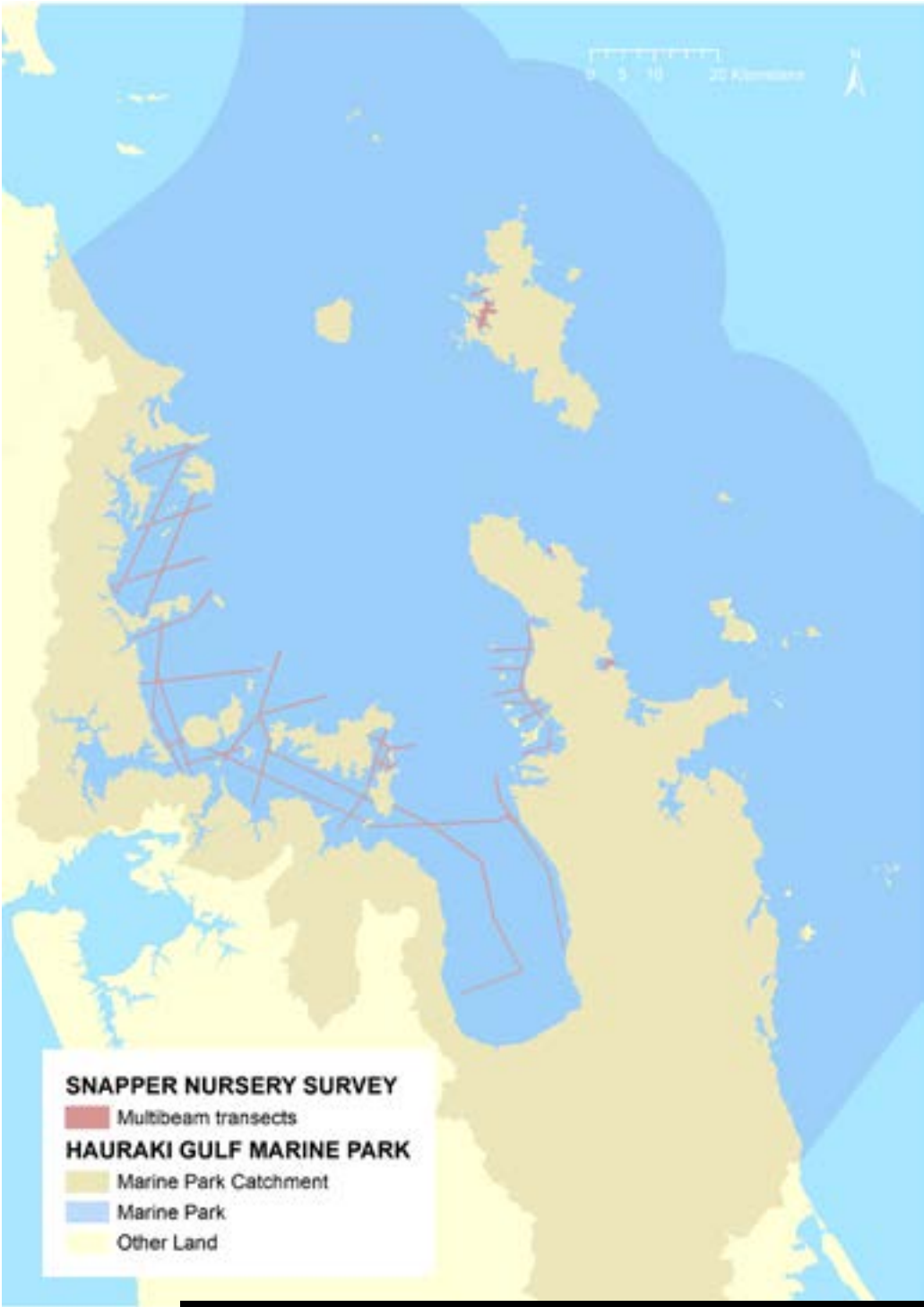
Figure 5.18: Multibeam sonar run-lines surveyed during a NIWA study on snapper nurseries (data provided by M. Morrison, NIWA).
