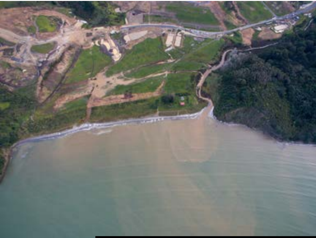
Figure 6.15: Sediment from an earthworks site and upper catchment adjoining Karepiro Bay, on the northern side of Ōkura Estuary. Photo by Geoff Reid.
